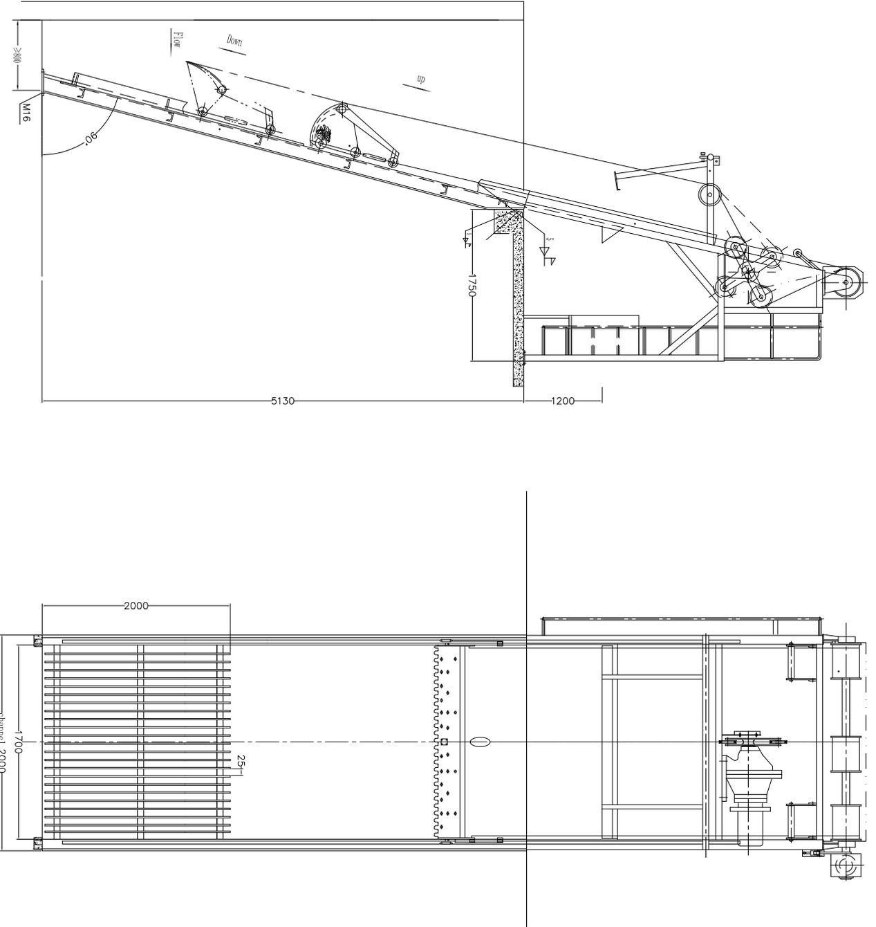
**cable operated grab screen(03 cables with rake)**
