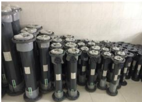
PVC pipe static mixer
