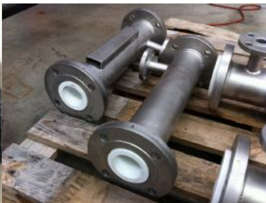
pipe static mixer with lining plastic
